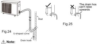
(1) The through-wall height of drain hose shouldn't be higher than the outlet pipe hole of indoor unit.(As show in Fig.25)
