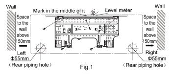
(2) Open a piping hole with the diameter of  $\Phi$ 55mm on the selected outlet pipe position.In order to drain smoothly, slant the piping hole on the wall slightly downward to the outdoor side with the gradient of 5-10°.(As show in Fig.2)
